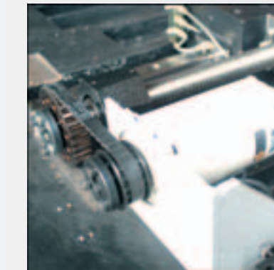
Backgauge positioning by AC Servo motor for high precision and maintenance free operation.
