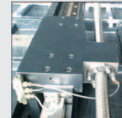
Precision motion control of backgauge: Linear motion bearings with hardened ground linear ways and precision ball screws with zero backlash enable smooth motion at upto 300 mm/sec.
